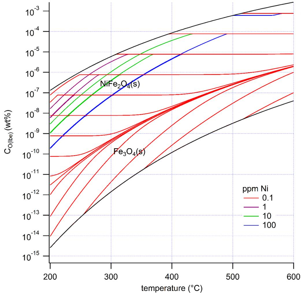
Trapping by precipitating  $\text{Fe}_2\text{NiO}_4$  in cold trap
