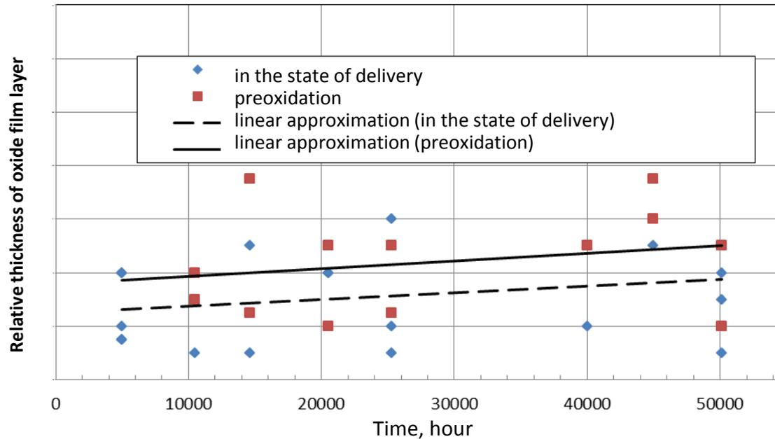
Bench corrosion testing of fuel rod models in the flow of coolant lead-bismuth was carried out on two identical loops SM-1 and CU-2M in the SSC RF-IPPE at the design values of the dissolved oxygen concentration and maximum circulation velocity of the alloy
