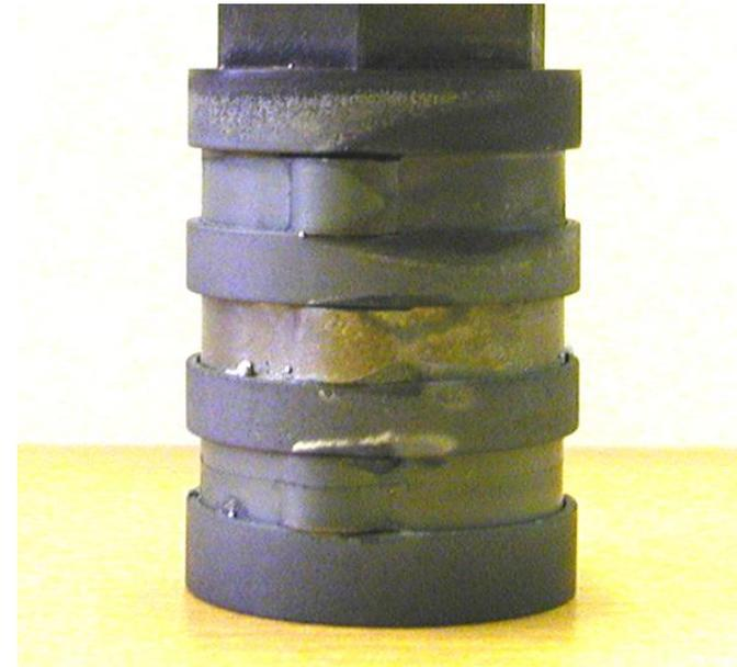
A view of the location of the cavitation zones behind the protrusions on the erosion samples after tests in lead at 1200 rpm and 650°C
