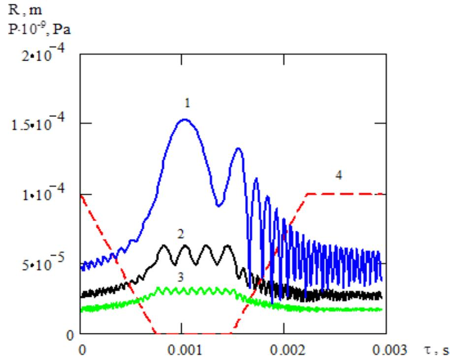
Change in the radius of gas bubbles in lead for a time ( $R_0$ : 1 – 50  $\mu\text{m}$ ; 2 – 30  $\mu\text{m}$ ; 3 – 20  $\mu\text{m}$ ) with the pressure change in the liquid (curve 4);  $\frac{dP}{d\tau} = 14 \cdot 10^7 \text{ Pa/s}$
