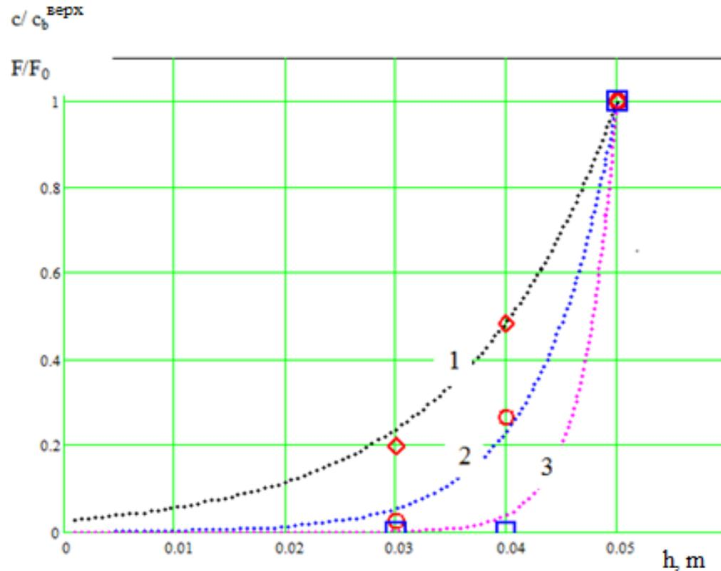
Distribution of the relative concentration of bubbles in lead by the crucible height at different rotational speed of the cylinder with the samples (curves):
