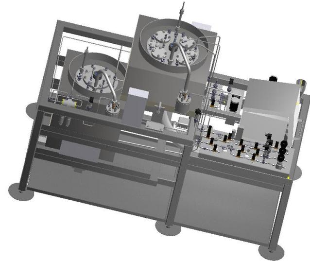
The facility consists of two cylindrical tanks, measuring tank and dump tank, and connecting piping to transport lead between the tanks as well as to deliver and extract gases to and from the facility, respectively.
