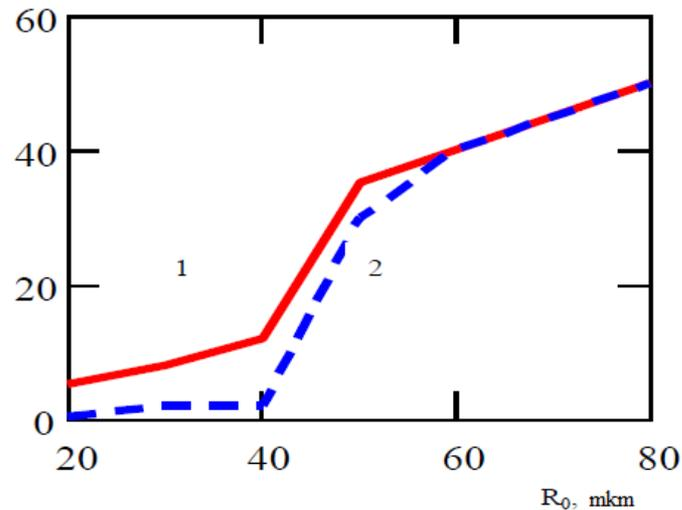
Dependence of the impact pressure of cavitation jets on the size of gas bubbles:
