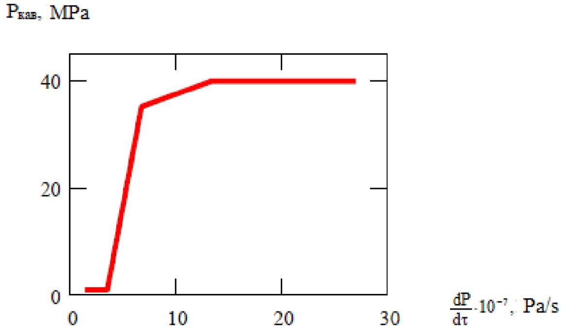
Dependence of the impact pressure of cavitation jets on the rate of pressure change in the lead for  $R_0=50 \mu\text{m}$
