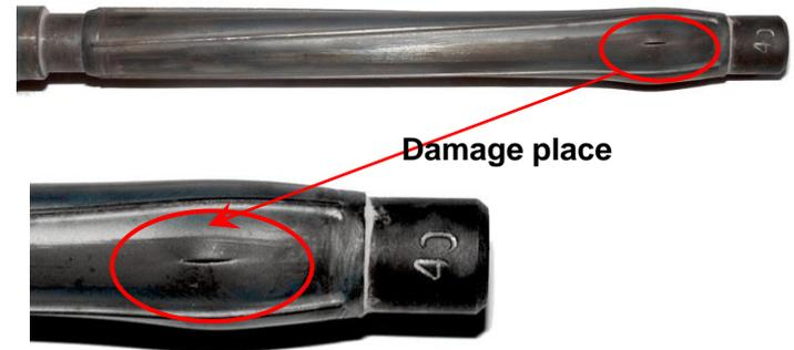
Typical view of samples after brake down tests (Sample №40 –  $t=850^{\circ}\text{C}$ ,  $\sigma=60\text{ MPa}$ ,  $\tau=9,5\text{ min}$ )
