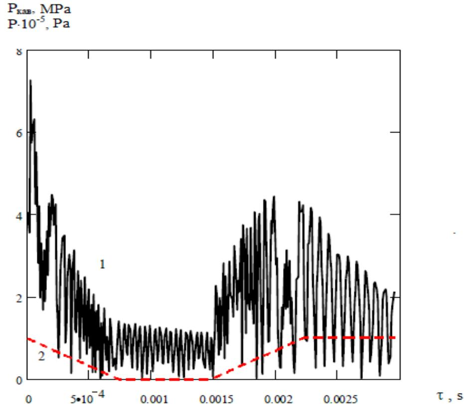
Pressure developed by lead jets on the wall for a bubble  $R_0 = 20 \mu\text{m}$ :
