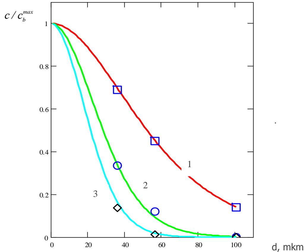
The relative concentration of gas in lead for different bubble sizes:
