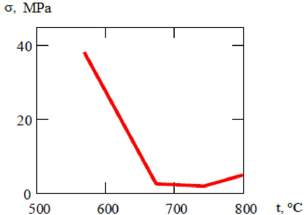
Dependence of the strength of iron oxide on temperature
