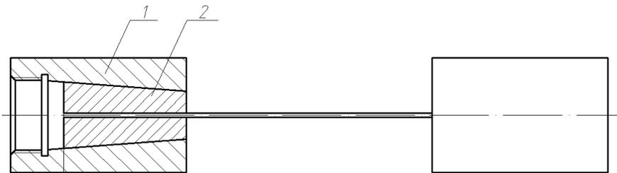
•1-liner, holding the sample; 2-hollow cylinder connecting to the rod of the test machine
